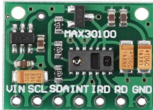
Fig 2. Pulse Oximeter Sensor
