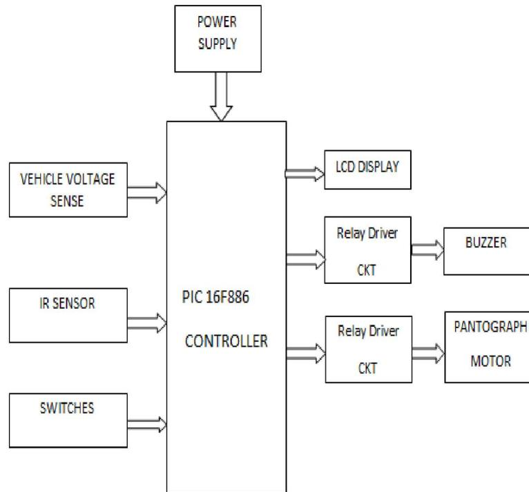
Fig. 2. Block Diagram (Charging Station unit)
