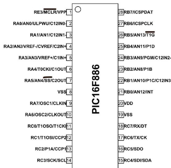
Fig. 4. PIC 16f886 microcontroller
