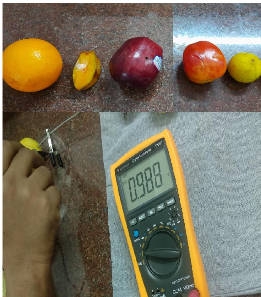
Figure 2: Fruits used for the study and measurement of cell potential
