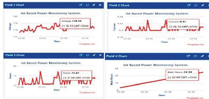
Fig. 4: Electrical measurements (voltage, current, power, and energy consumption) of load.
