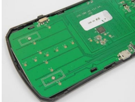
Figure V: The horizontal traces, test pads, and various horizontal traces of PCB
